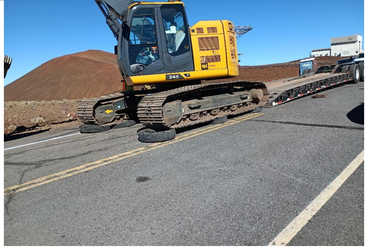
^ 8:33am - loading excavator onto lowboy
