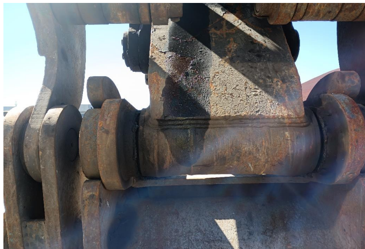
^ 3:05pm - oil spot at bucket with witness mark
