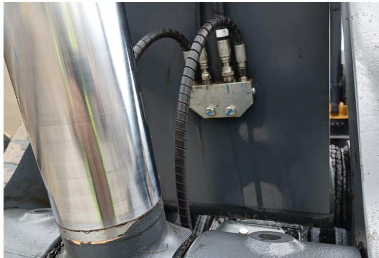
^ 1:29pm - leaking hydraulic block
