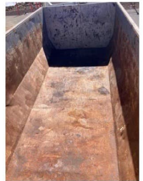
1233: Hydraulic oil in bed of truck. *SOURCE OF SPILL
