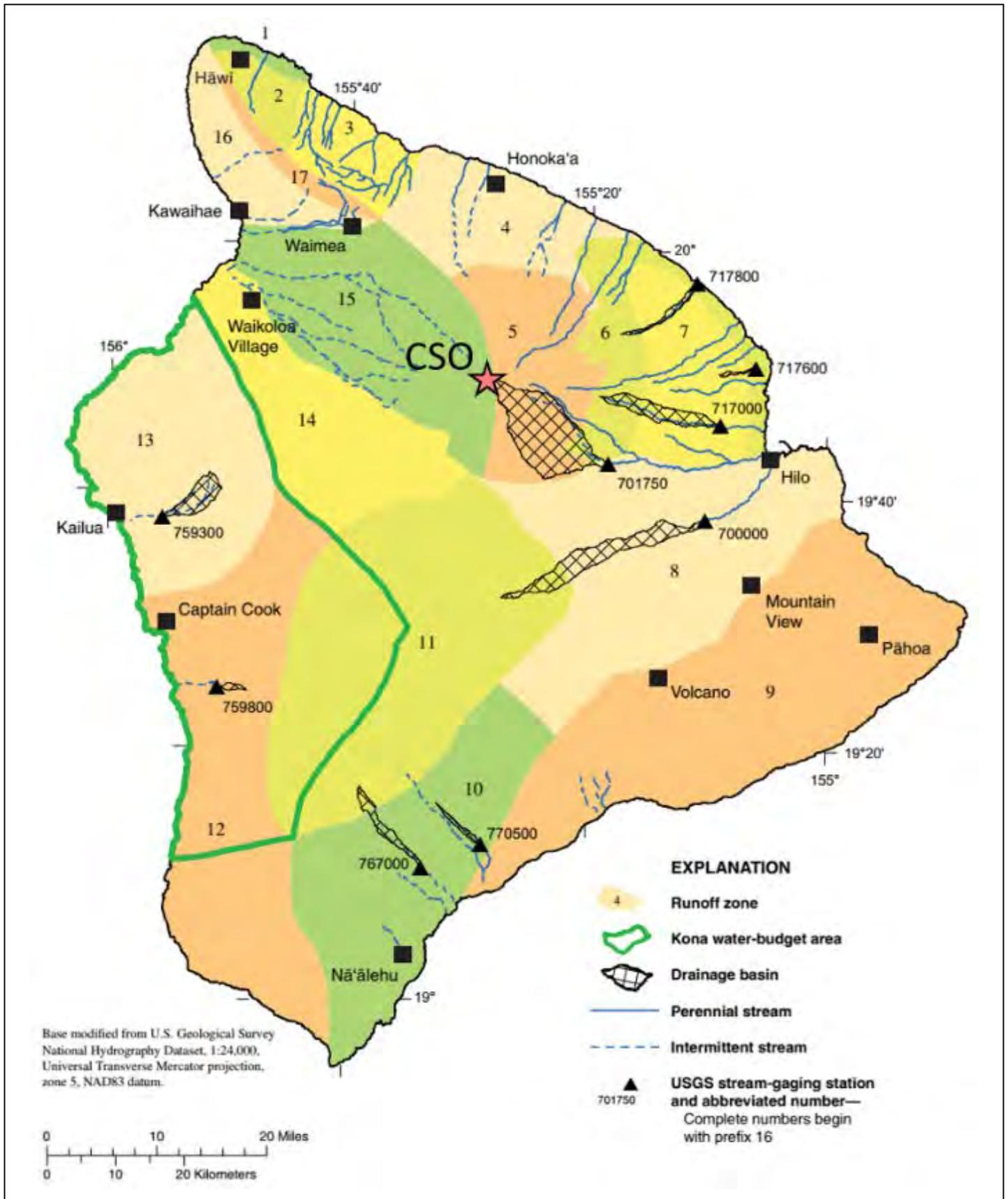
**Figure 16. Zonation Used for Hawai'i Island Water Budget by the U.S. Geological Survey (Engott, 2011).**
