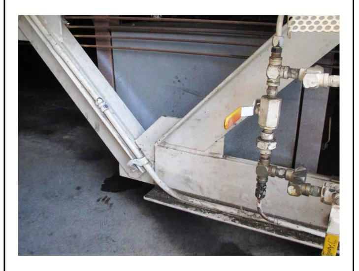
Photo 15Minor Fluid Leak Under the First Level Platform
