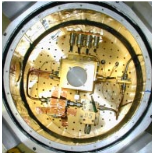
Fig. 12. Cryostat cold surface. The RF and LO signals enter from above, go through the polyethylene lens in the center, and enter the mixer block. The IF signal goes out the coax cable to the left, through the isolator (under copper tape), through the LNA, and out the dewar to the upper right.
