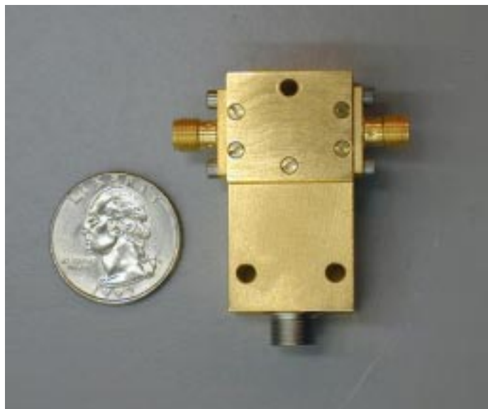
Fig. 5. The assembled amplifier. The lid between the SMA connectors covers the microwave cavity.
