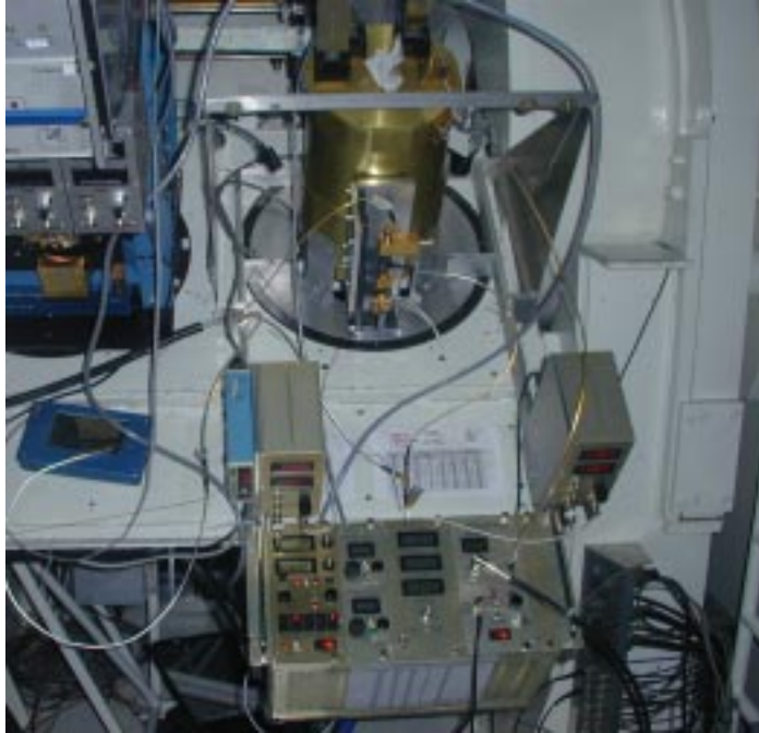
Fig. 15. Receiver mounted at the Cassegrain focus of the CSO. The receiver is in a downward-looking cryostat at the top of the photo. The 690 GHz LO chain is on the front of the cryostat. The rack at the bottom of the photo houses, from left to right, the SIS bias box, magnet bias box (for Jospheson oscillation suppression), LNA bias box, and 4 to 8 GHz IF system.
